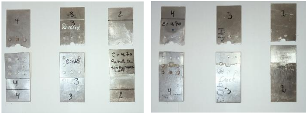
Fig.24. Damage to the notched plates repaired by an aluminum patch using hybrid repair processes (bonding/riveting).
