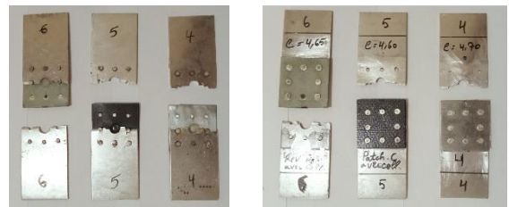
Fig.27. Damage to the notched and cracked plates repaired by different types of patches using hybrid repair processes (bonding/riveting).
