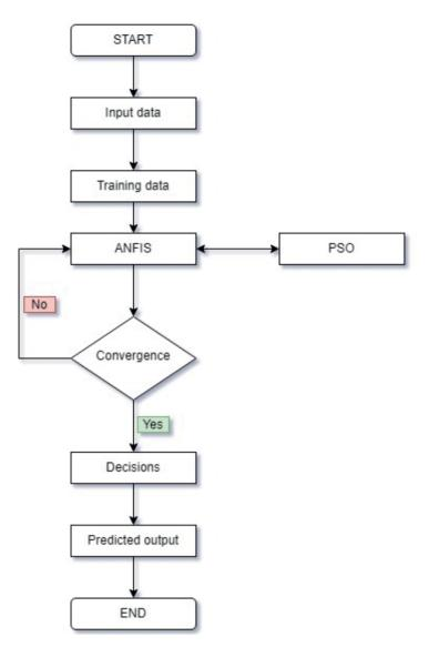
Fig. 3 - Diagram of the optimised ANFIS using the PSO algorithm.
