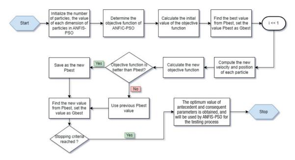
Fig. 2 - Diagram of the applied PSO algorithm workflow.
