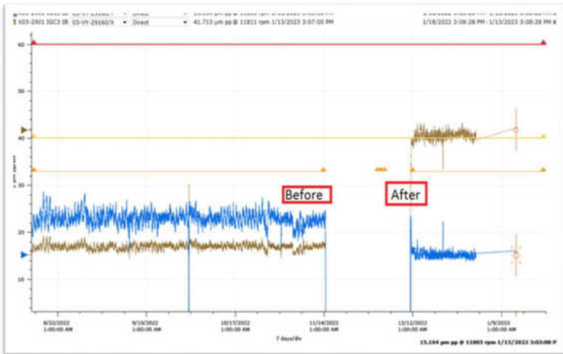
Figure V.34 : LP compressor vibration drive end
