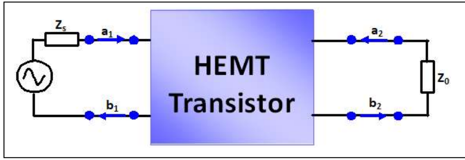
Figure I.18 Quadripole representation, adapted from [52].
