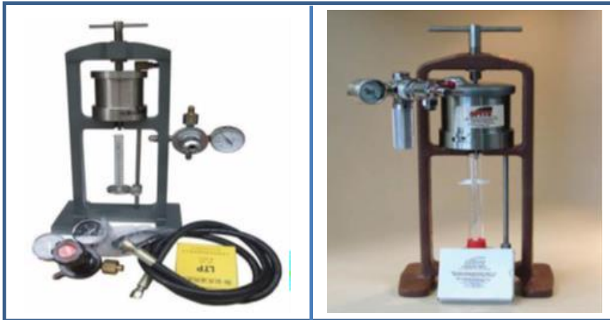
Figure I.4: Filtre-presse API, Filtre-presse haute pression haute [8].
