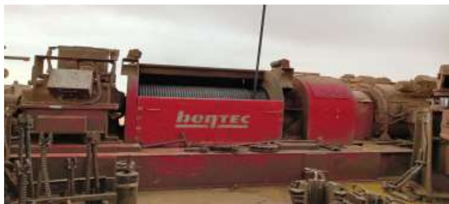
Figure I-7: Treuil de forage
