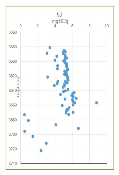
Figure 14: Profile of variation of residual potential S2 as a function of depth in the well Z-1
