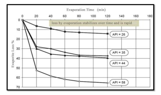
Figure 21: Graph shows the loss of hydrocarbons over time according to Noble R et al (1997)
