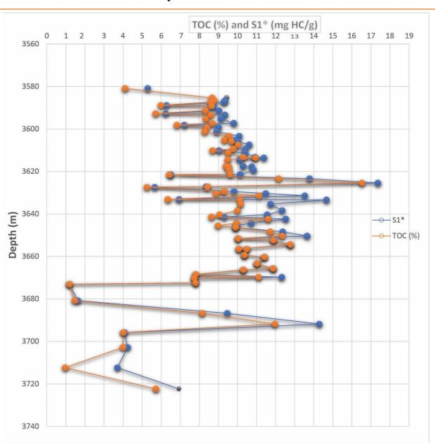
Figure 23: Free potential variation profiles corrected and TOC as a function of well depth Z-1.
