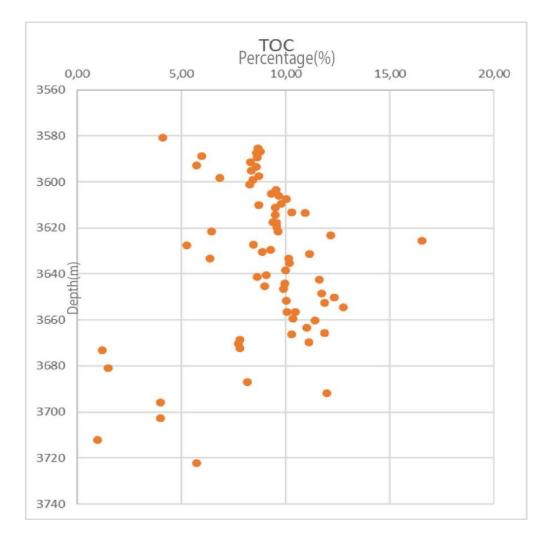
Figure 12: TOC variation profile as a function of depth in wells Z-1
