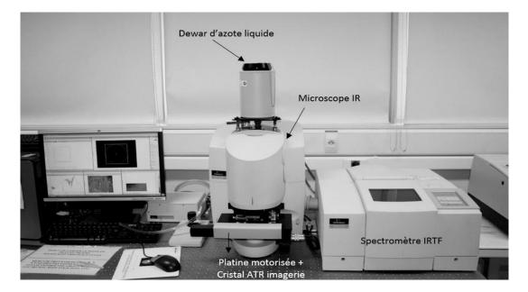
Figure 10: Photometric microscope coupled to a spectrometer (As and Co.)
