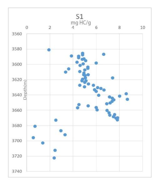
Figure 13: Free potential variation profile S1 as a function of depth in the well Z-1
