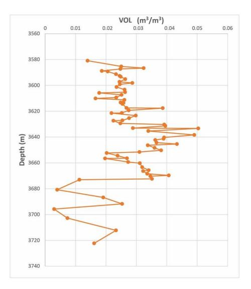
Figure 25: Hydrocarbon volume variation profile as a function of well depth Z-1.
