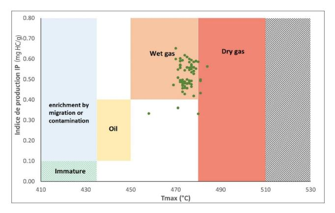
Figure 15: Maturation diagram according to IP and Tmax of Z-1 well.
