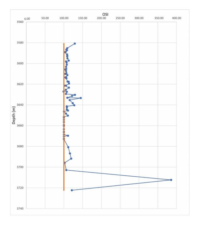
Figure 24: OSI oil saturation index variation profile as a function of Z-1 well depth.
