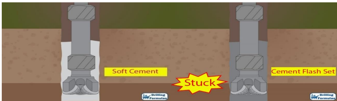
Figure II-6. Ciment mou (Soft Cement). (DF,2011)
