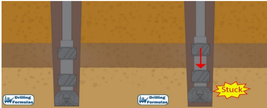
Figure II-14. Under gauge borehole. (DF,2011).
