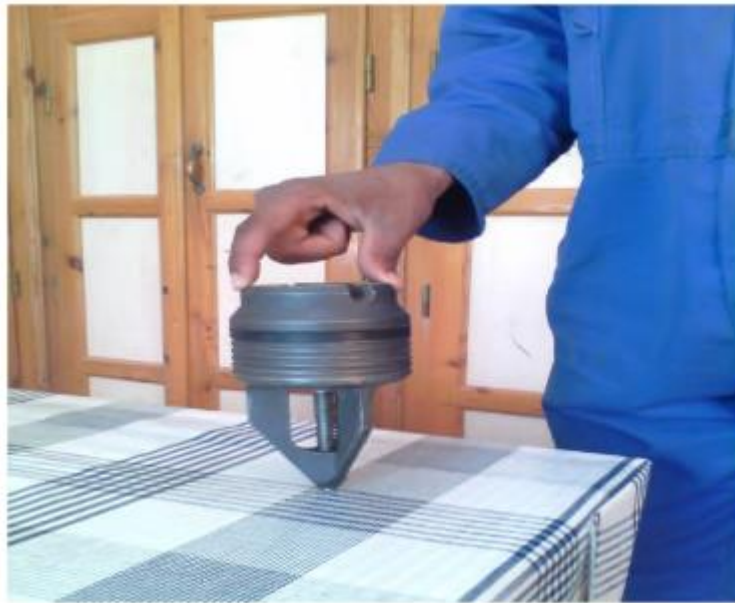
Figure V.4 : la BPV (back pressure valve).
