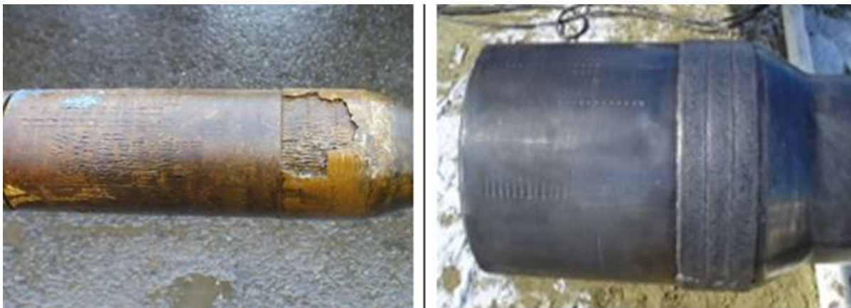
FIGURE 3.5 – Tool joint hardbanding
