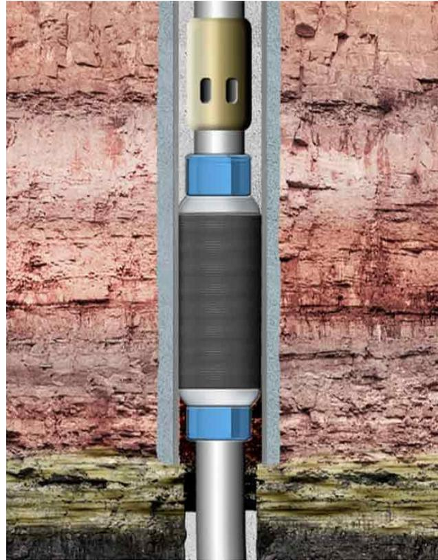
Figure A.III. 10: External Casing Packer (ECP)
