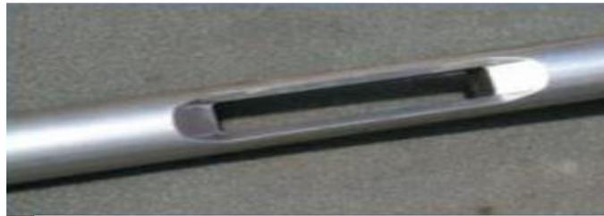
Figure A.IV.18: Gradiomanometer
