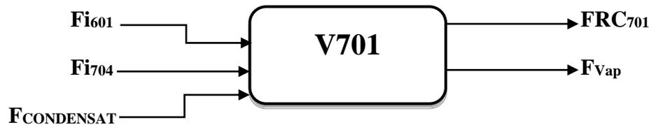
$$F_{i601} + F_{i704} + F_{\text{Condensat}} = F_{\text{RC701}} + F_{\text{Vap}}$$
