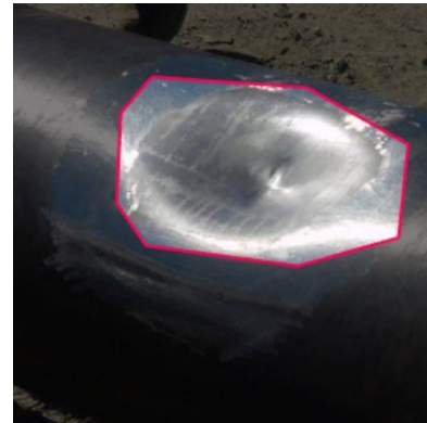
Figure 0-2: segmentation of a dent
