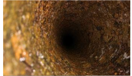
Figure 1-4: Endoscope Cameras view inside a pipeline
