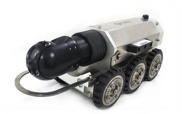
Figure 1-1: industriel pipe inspection crawler camera robot
