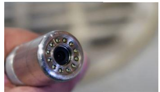
Figure 1-3: Push Rod Cameras:
