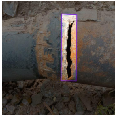
Figure 0-3: segmentation of a crack
