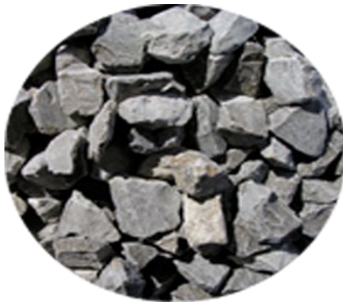
Figure I.13. Gravier Ballast 25/50 mm
