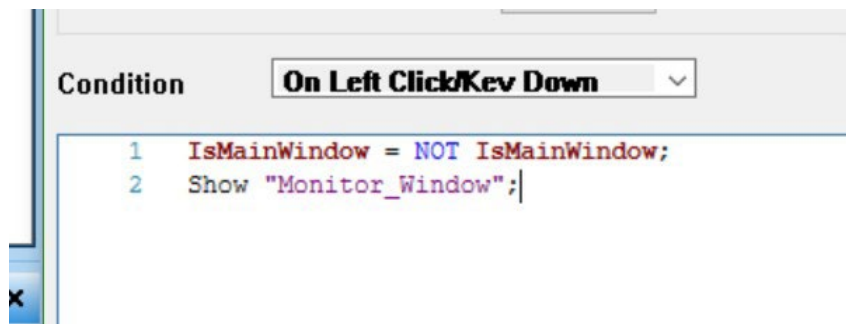
Figure 5.5: Navigation script for a button for switching between windows in Aveva InTouch HMI
