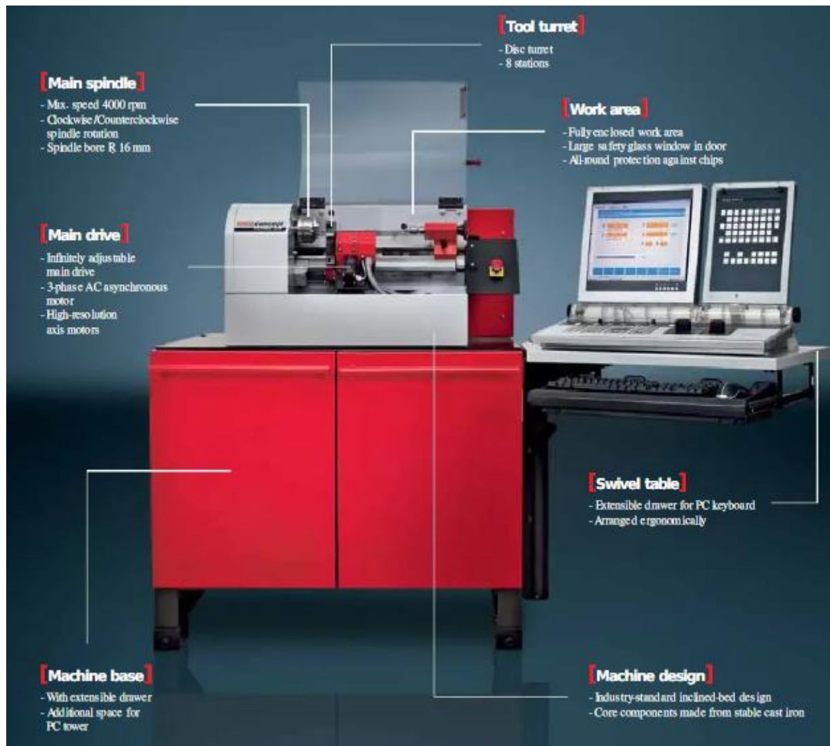
Figure IV.1: EMCO Concept TURN 55 with description. [13]
