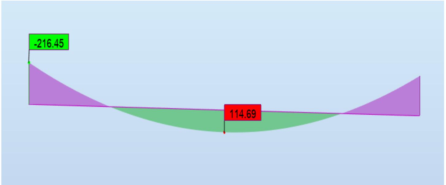
*Figure V 5: Diagramme des moments fléchissant à l'ELS.*
