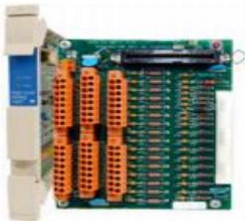
**Figure 3.11** : FTA (Field Termination Assembly)
