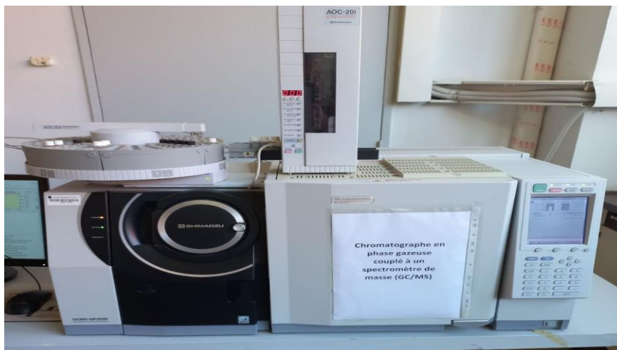
Figure 16 : gas chromatography device coupled to a mass spectrometer (GC/MS)
