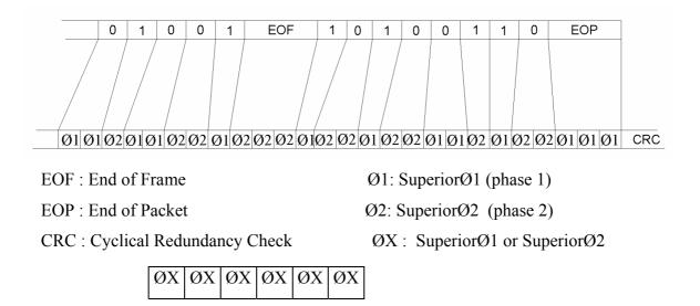
Cyclic Redundancy Check. Cyclic redundancy checking uses a division operation on the transmitted sequence, appending the remainder of the division operation to the message transmitted. At the receiver, this same operation occurs. If the result of the division is other than zero, an error has occurred. CRC error checking methods have very high detection percentages (more than 90%), but are very demanding in terms of computation time.
