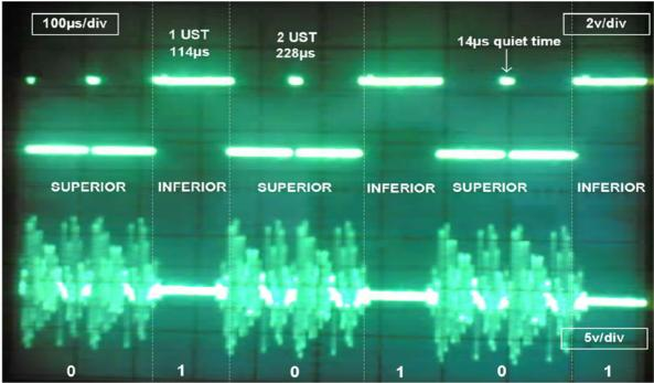
Figure 5.5 Preamble Transmission of 010101
