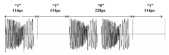
Figure 3.3 Amplitude Shift Keying (ASK) Data Pattern
