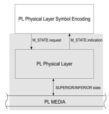
Figure 3.7 Powerline Lower Layers Relationship [22]
