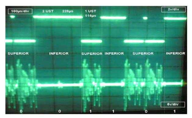
**Figure 5.6 Preamble Transmission of 001101**
