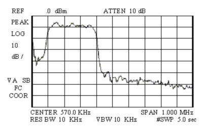
Figure 3.2. Frequency Spectrum of a PL "Chirp" [1]
