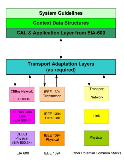
Figure 4.4 Application Diagram Supporting HomePnp on Multiple Stacks.
