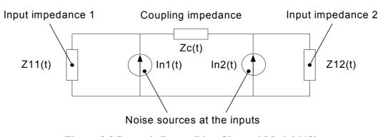
Figure 2.2 Dosert's Power Line Channel Model [18]
