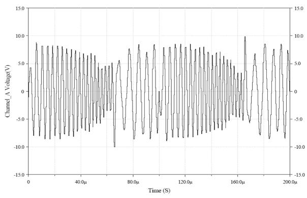
Figure 5.4 transmission of two consecutive "1" in a packet message.
