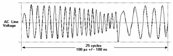
Figure 3.5 Frequency Swept Carrier Waveform
