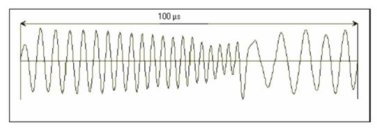
Figure 3.1 Spread Spectrum Carrier Chirp
