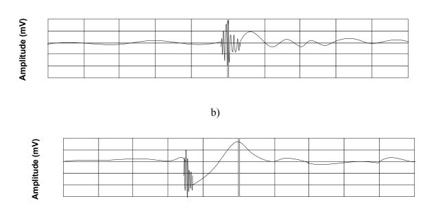
Figure 2.1 One sample of impulsive noise generated by a) an electrical drill b) a light dimmer [2].
