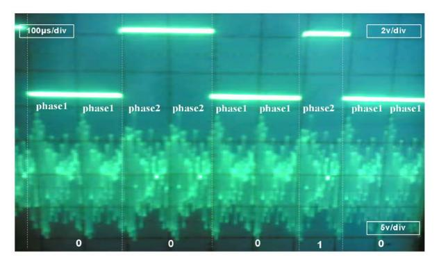
Figure 5.7 Packet Transmission of 00010
