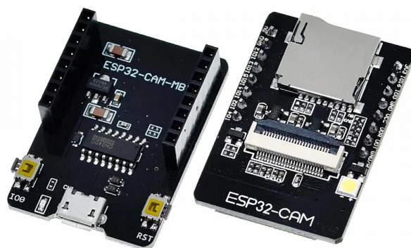
Figure 4.3: ESP32-CAM-MB USB-to-UART converter, and the ESP32-CAM board.
