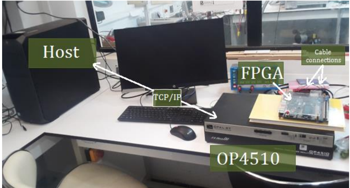
Figure II-20: The Final Hardware Setup of the experiment.
