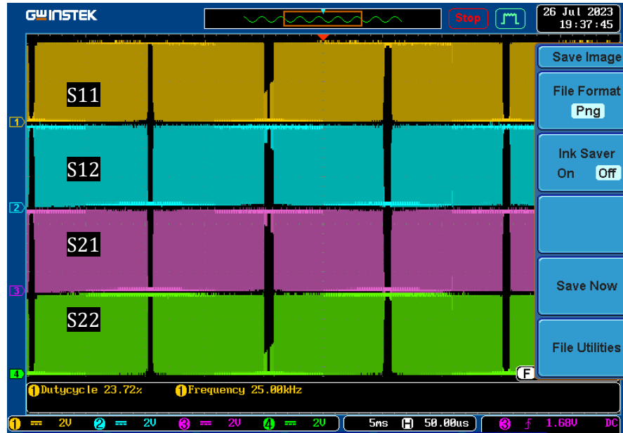
Figure III-18: Gating signals generated from the FPGA-Based controller
