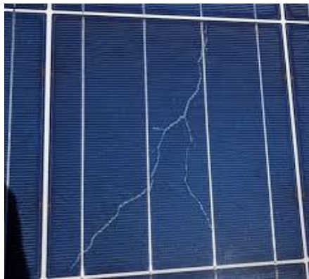
Figure 2.7: Snail trail effect on a PV module
