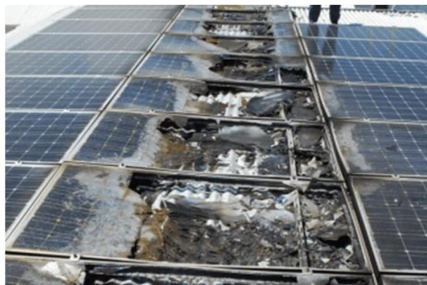
Figure 2.11: Damaged PV system due to an Arc fault
