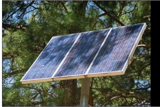
Figure 2.2: Partial shading on a solar module
