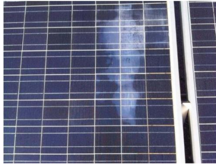
Figure 2.6: Delamination effect on a PV module
