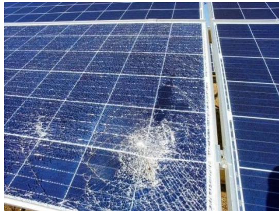
Figure 2.3: Cracked solar module
