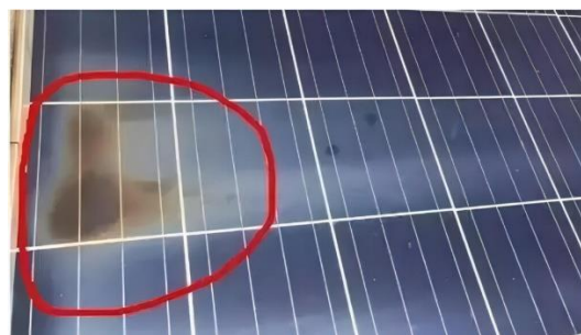
Figure 2.1: Hotspot in a PV panel
