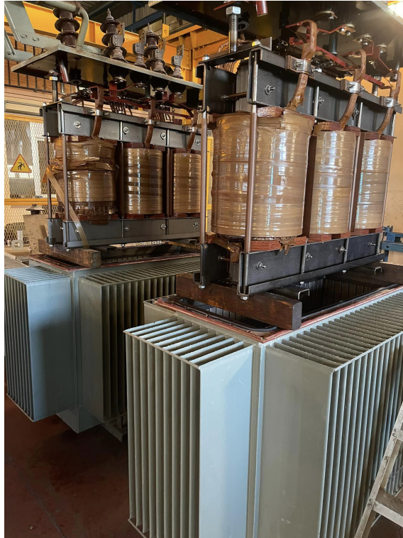
Figure 58. Active part of a distribution transformer
