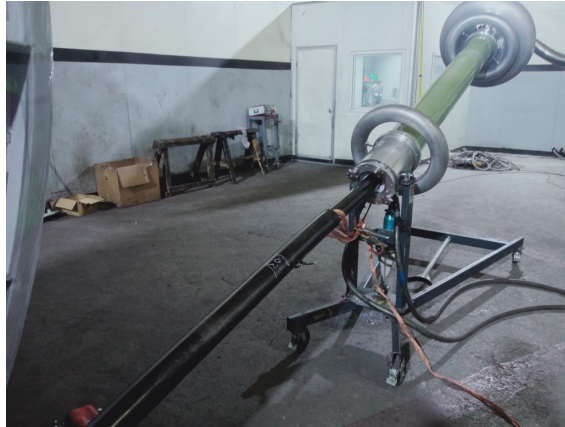
Figure 66. Connecting the cable to the water pumping termination
