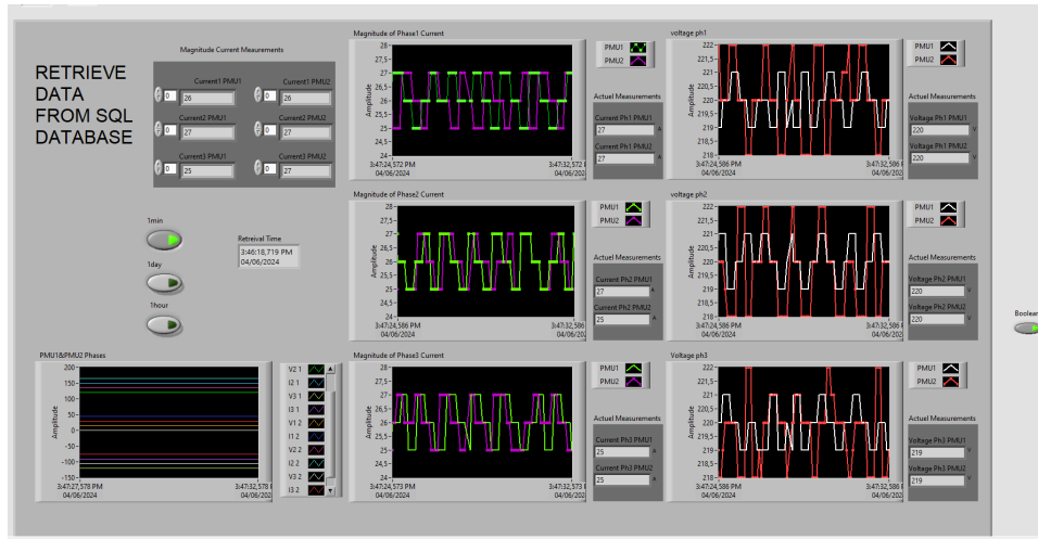
Figure IV.19: Retrieved 1min data chart with time alignment
