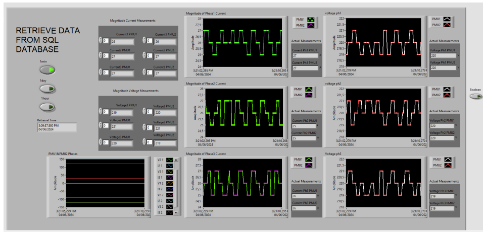
Figure IV.15: Retrieved 1min data with no time alignment chart(False case)
