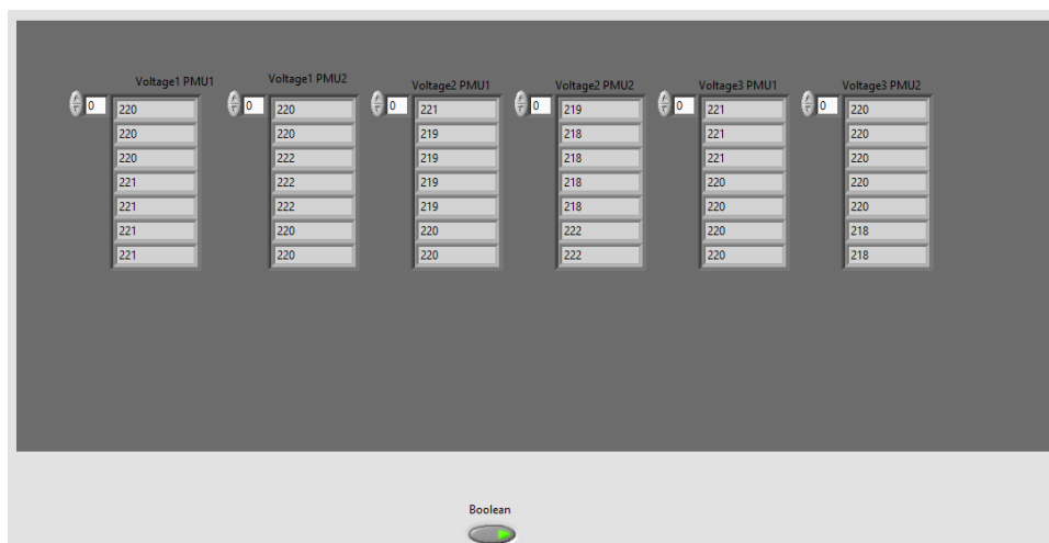
Figure IV.18: Retrieved 1min data with no time alignment array(False case)
