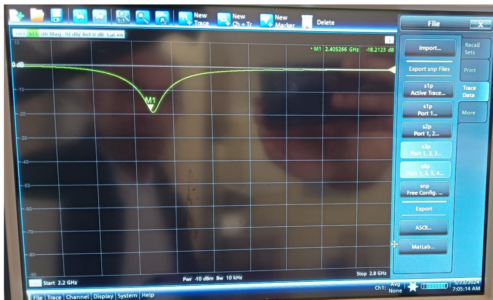
Figure 4.5 Input reflection coefficient level for the antenna using vector network analyzer
