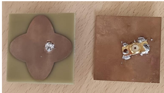
Figure 4.1 Fabricated patch antenna front view (left) and back view (right)
