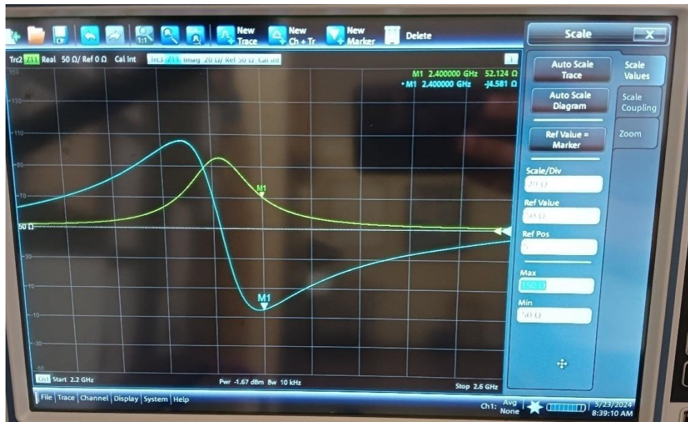
Figure 4.4 Antenna input impedance measurement using vector network analyzer
