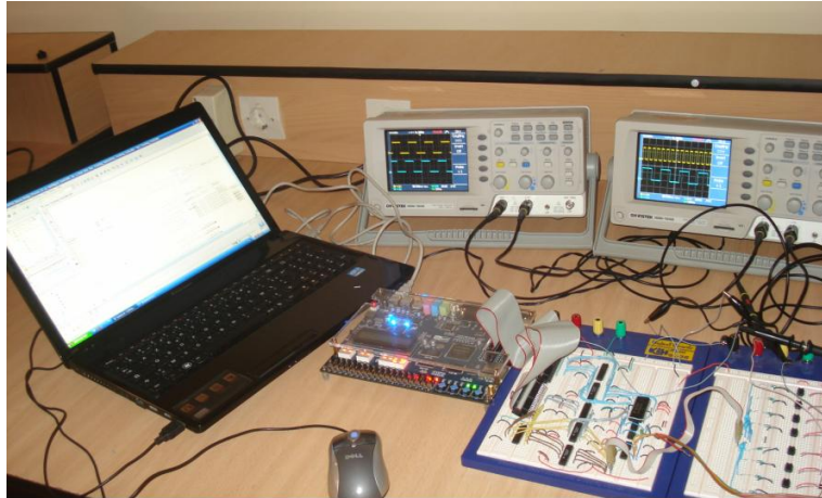
Figure-6.16. (b). Hardware setup of the FPGA-based intelligent dual-axis sun tracking system.
