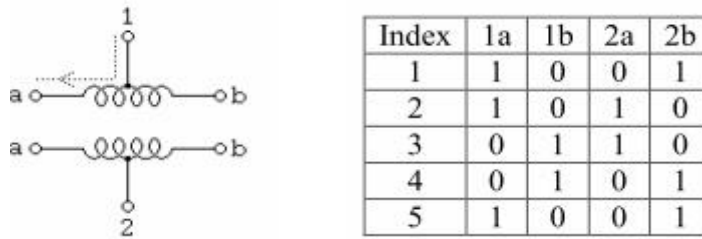
Figure 6.11 Unipolar stepper motor windings and full-step sequence.
