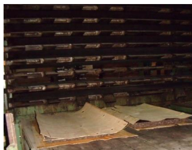
Figure V.3. Elaboration des panneaux sandwiches.
