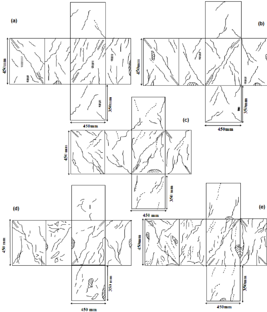
Fig. 2. Schema of the location of cracks in rock samples after the experiments in dry strain conditions: granite (a), marble (b), diabase (c), pyrophyllite (d), and concrete (e).
