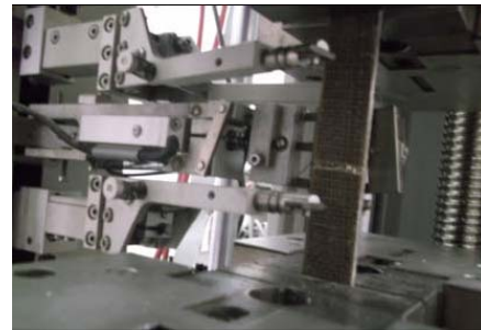
Fig. 7 Rupture in traction of the laminate
