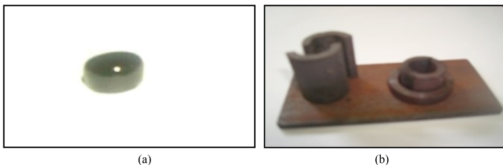
Fig. 1 Pictures of (a) the fabricated nuclear glasses and (b) the casting mould.
