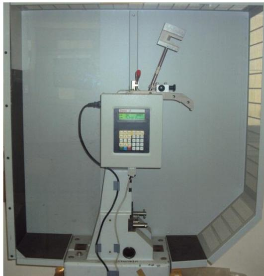
Figure III.12 : Appareil Choc Charpy.
