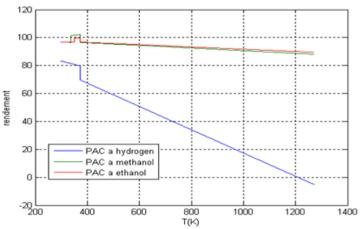
Figure 9 : Influence of temperature on the reversible yield of FC (P = 1atm Pure Oxygen)
