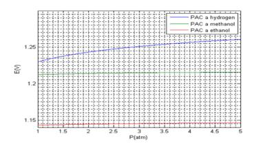
Figure 7 : Effect of the pressure on the EMF of FC (T=298K pure oxygen pure)
