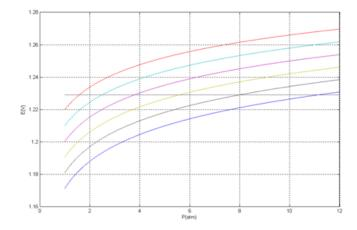
Figure 8 : The compensation pressure at different temperature values for FC with hydrogen (E = 1.23V)
