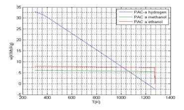
Figure 11 : Influence of temperature on the energy density of FC
