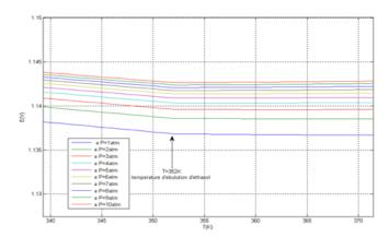
Figure 10 : Effect of the temperature on the EMF of ethanol FC for different pressure values (T=298K a T=370K)
