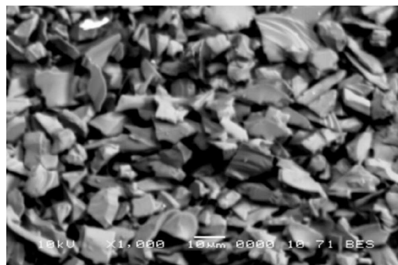
Fig. 2. The SEM morphology of as-received 7 μm average particle size SiC powder.
