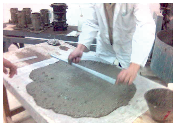
Fig. 8 Slump flow test by Abrams cone
