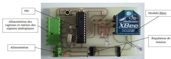
Figure 5.6 carte d'acquisition comportant la technologie XBee
