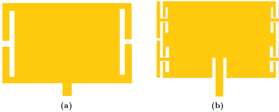
Figure 2.11: DMS :(a) Simple spur-line[29] and (b) Slots with spur-line [30]
