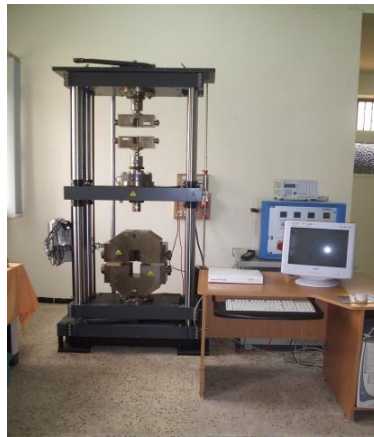
Figure 3.5 – Machine universelle de traction ZWICK 250/SN5A
