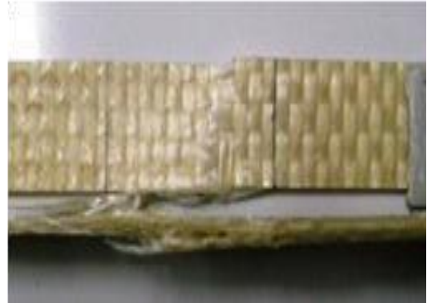
Figure 6. Breaking mode by tensile test of laminate
