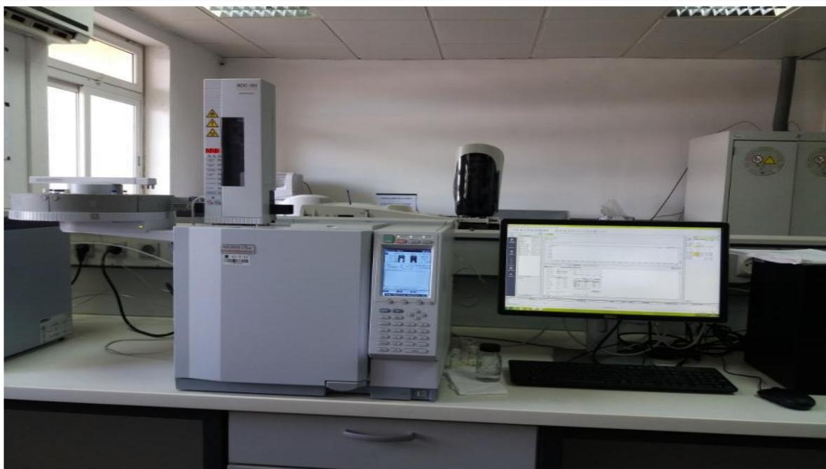
**Figure III.25:** Appareil CPGC (2010-plus SHIMADZ).
