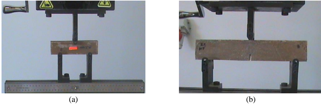
Fig. 1(a) PC flexural test set-up, and (b) PC fracture test set-up
