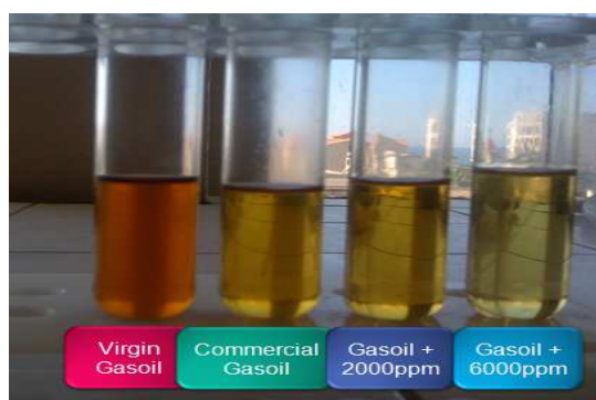
Figure 9. Colouring of Diesel oil after the tests with oxidation.
