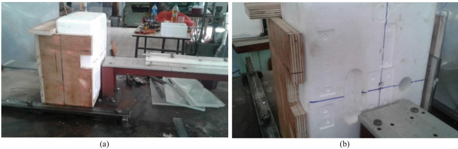
Fig. 5. Test bench for 200 m experiment: a) The projectile recuperator, b) The penetration position
