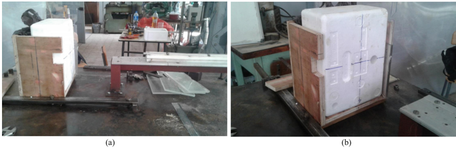
Fig. 6. The Test bench for 400 m experiment: a) The projectile recuperator, b) The penetration position
