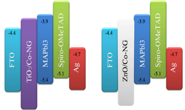
Fig. 6. Energy level diagram of the studied perovskite solar cells.
