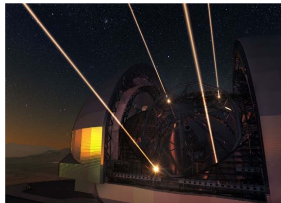
Figure 2. European Extremely Large Telescope's multi-LGSs system [6].
