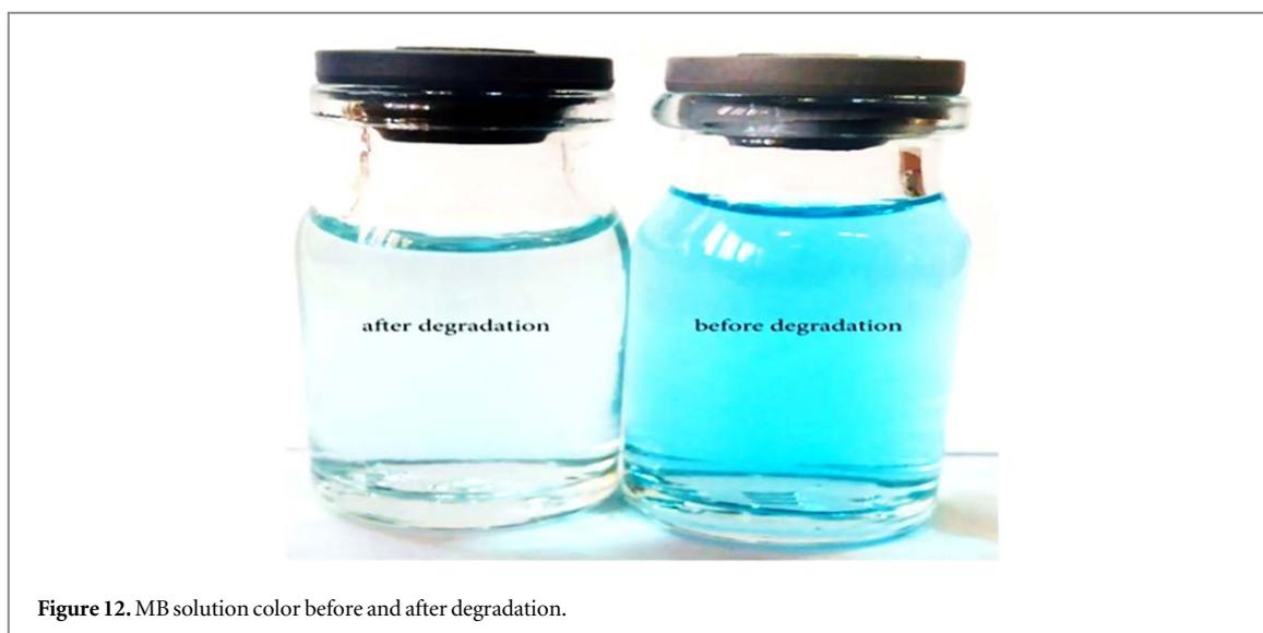
Figure 12. MB solution color before and after degradation.
