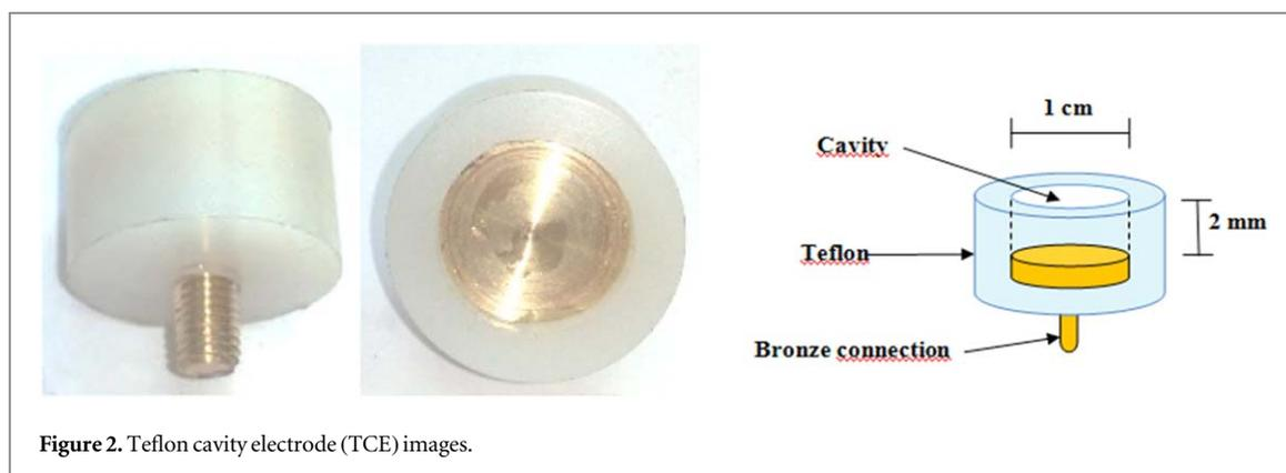
Figure 2. Teflon cavity electrode (TCE) images.
