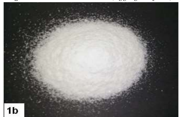
Figure 1b. Ground HDPE Grade 4903.
