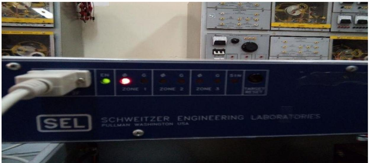
Figure 5.16: SEL 221 Tripping in Zone 1 for Case 02 Fault
