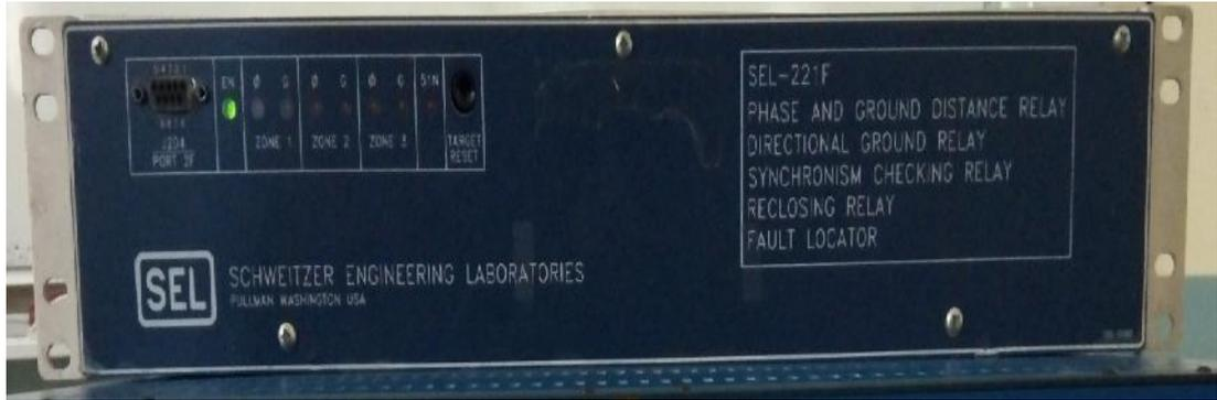
Figure 2.1: SEL-221F Numerical Distance Relay
