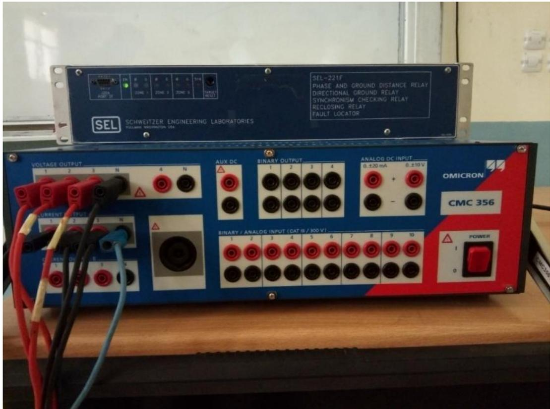
Figure 2.4: SEL 221 Relay and OMICRON CMC 356 Put Together In IGEE Lab Bench
