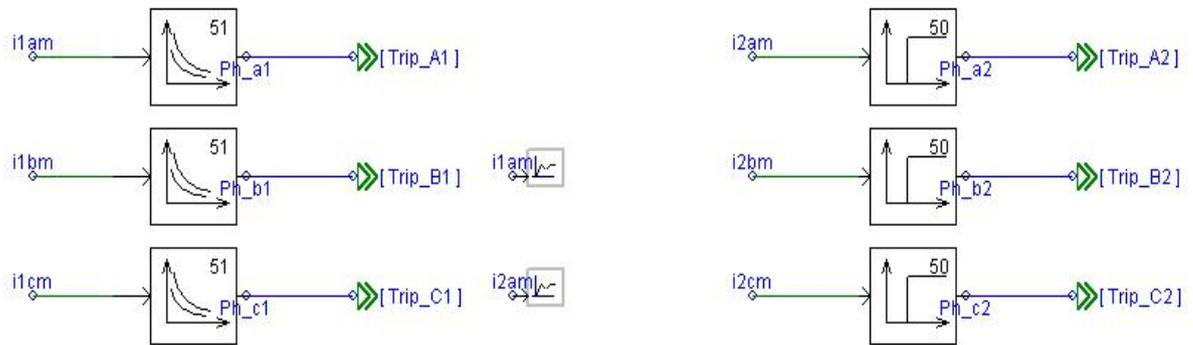
Figure 3.8: Overcurrent Relay Models
