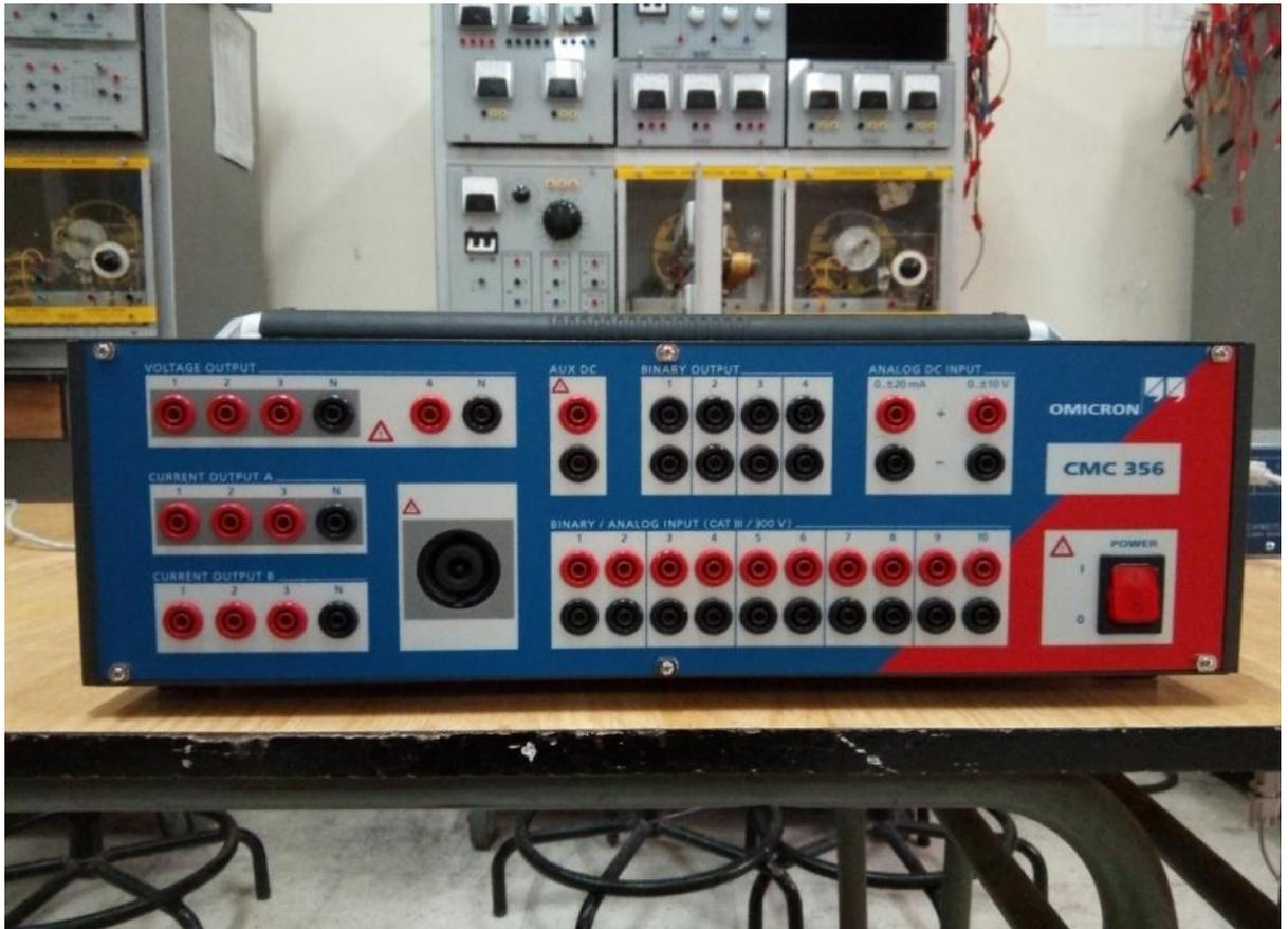
Figure 2.5: Injection Test Set OMICRON CMC 356
