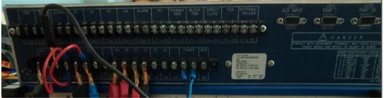
Figure 2.9: Rear View of SEL 221F Relay with Voltage and Currents Inputs Connected
