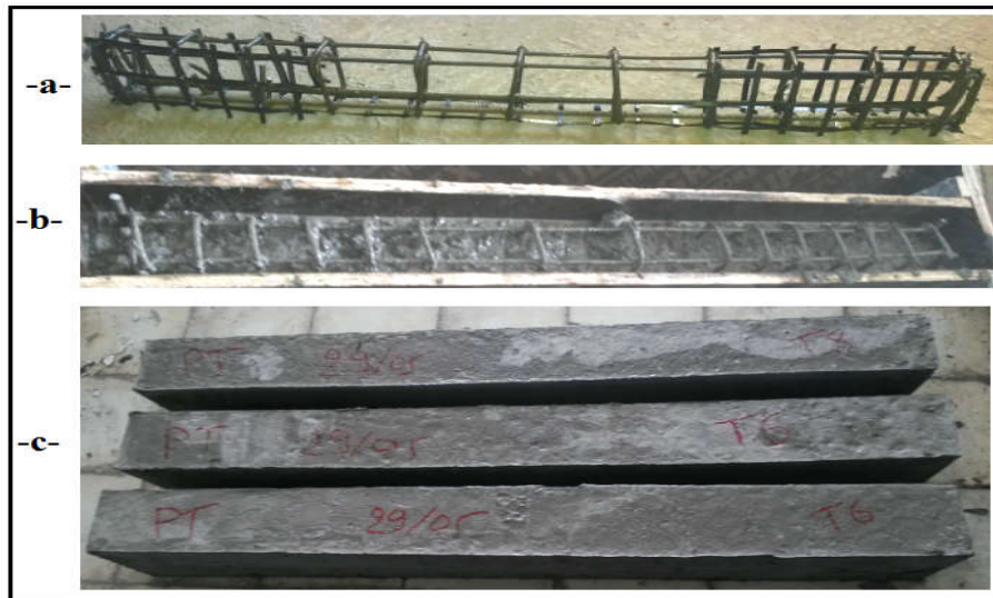
Fig. 4 Preparation of the RC beams strengthened by composite grids
