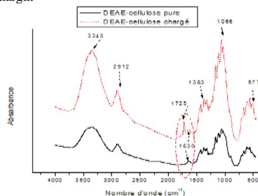
**Figure 3.** Infrared spectra of pure and charged DEAE-cellulose.
